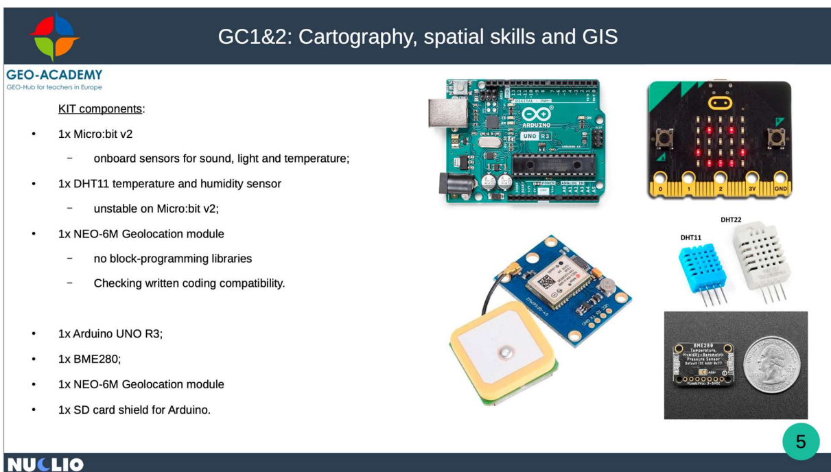
Figure 3: Components of the GC1&2 (Cartography, Spatial Skills and GIS) configuration of the GEO-Kit, including the Arduino UNO R3 and micro:bit controllers, temperature and humidity sensors, and GPS module.
