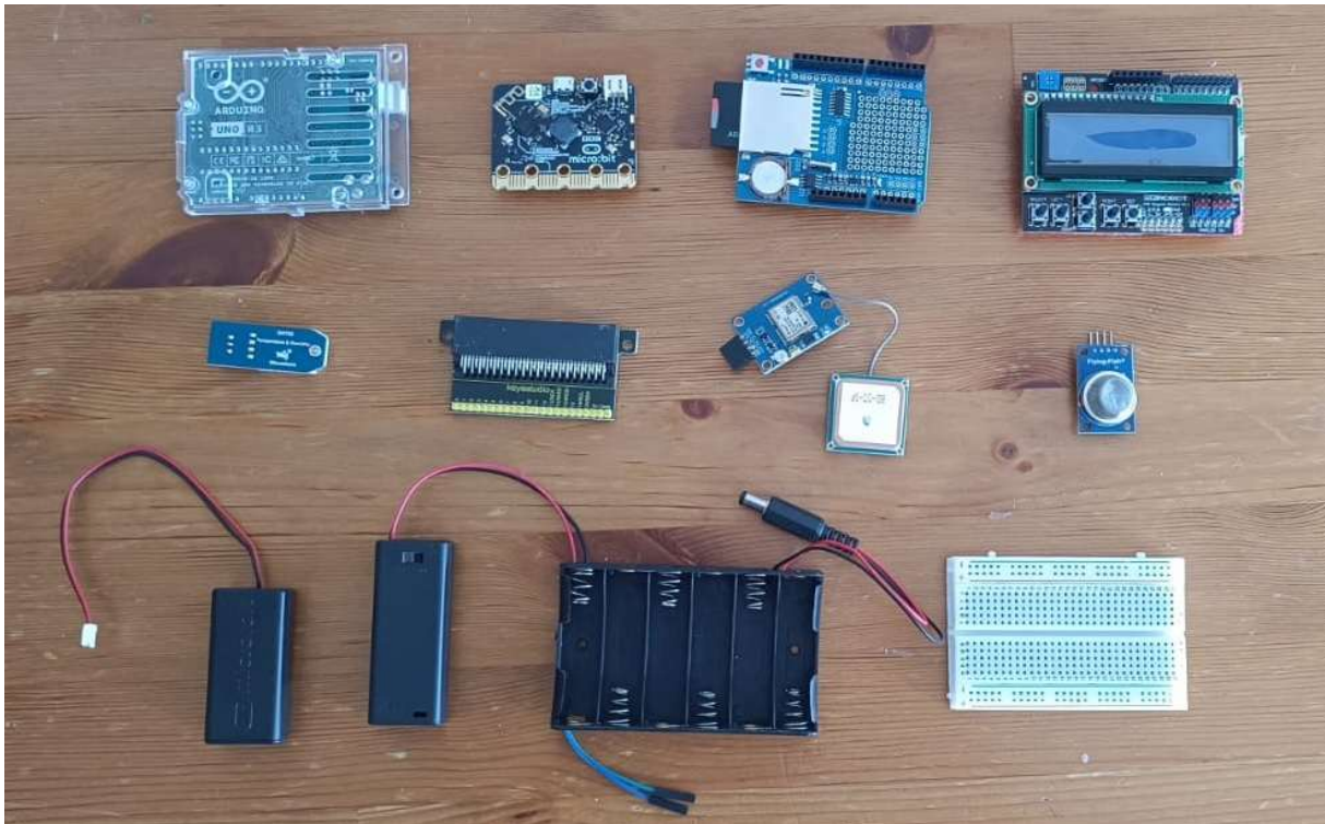
Figure 2: GEOKIT main electronic components. From left to right; top row: Arduino UNO R3, BBC Micro:bit (v2), Arduino SD card shield, LCD shield; middle row: temperature and humidity sensor, micro:bit extension board, Arduino GPS module, gas/dust/air quality sensor; bottom row: micro:bit battery packs, Arduino battery pack; breadboard.
